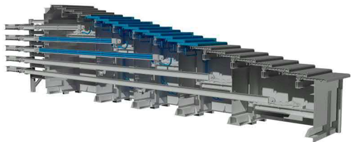
LAWI Water-Cooled Moving Grate
