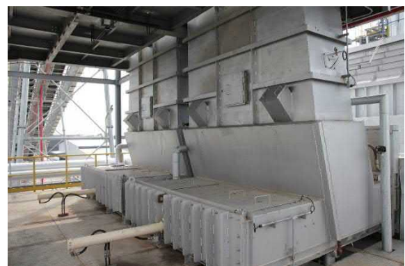
2-Lane Fuel Dosing System with Fuel Pusher
